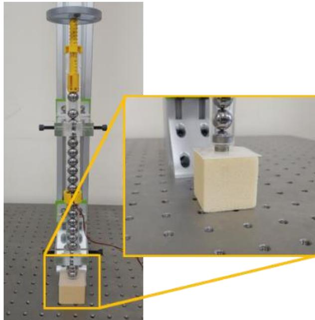
Fig. 1 Experiment Setup; the granular sensor consisting of 21 particles is placed on top of the PU foam covered with a silicon rubber layer.
